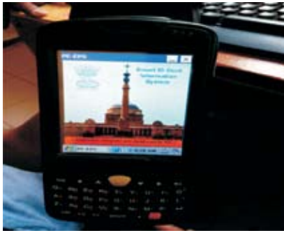
RFID Scanner to read Smart Cards issued to all the residents of President's Estate
